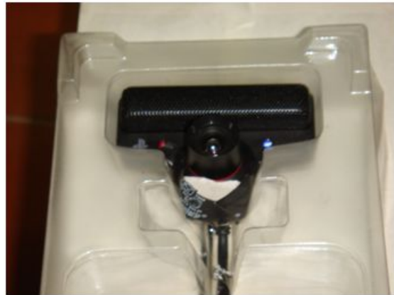
Figure 4.3: PS3Eye camera converted to IR camera
